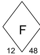
This blueprint label (diamond) designates the termination location of fiber cable(s). There are 12 single mode strands and 48 multimode strands terminated in this communication room
