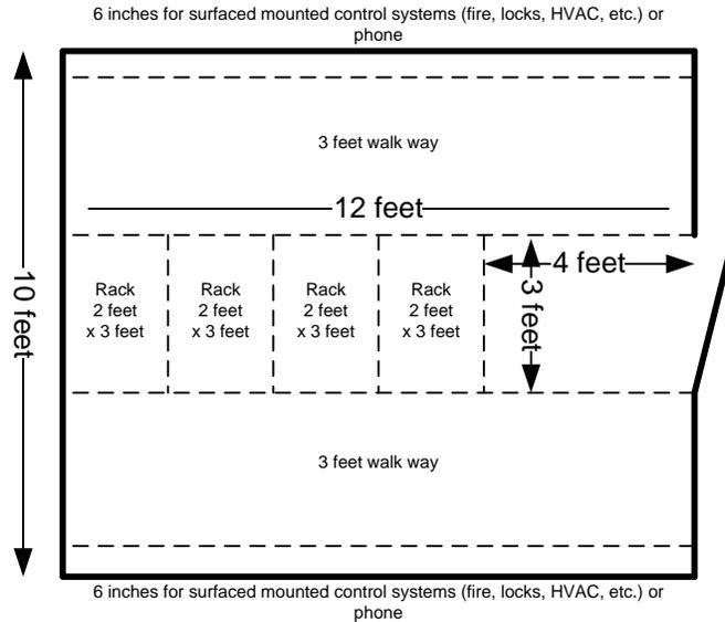
2.1.2.3.2. One secondary communication room should be centrally located on every floor
