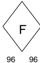
This blueprint label (diamond) designates the termination location of a major fiber building trunk because of the large number of strands. There are 96 single mode strands and 96 multimode strands terminated in this communication room
